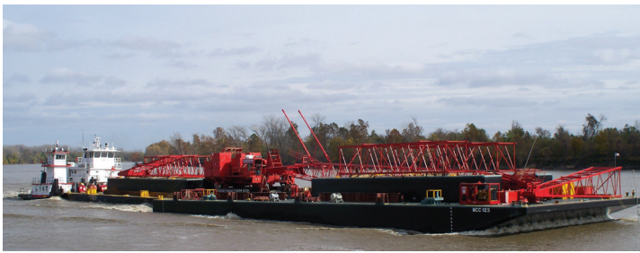
Manitowoc 7000 crane headed up the Missouri river for a Kansas City bridge job.
