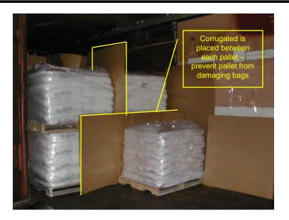
Boxcars were loaded from the bulkheads toward the middle of the car (to the doors). Note the application of AK board between the product, thus providing a smooth surface for each pallet in the boxcar. Boxcars were loaded from the bulkheads towards the middle of the car (to the doors).
