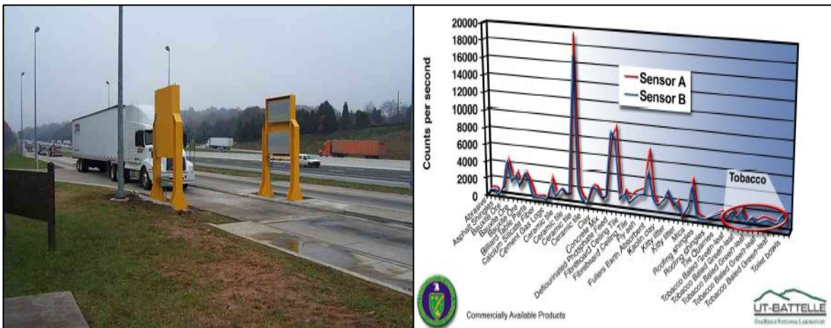
Figure 7: IMRicS System and Cargo Representation of Radiological Signatures (4)
