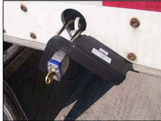
Figure 5: E-Seal Attached to Freight Trailer (5)
