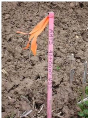
Figure 8. Oconto Bypass Slope Stake Lath Marked with Identifier, Station, and Offset
