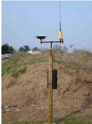
Figure 3. River View's Base Station atop a Permanent Post
