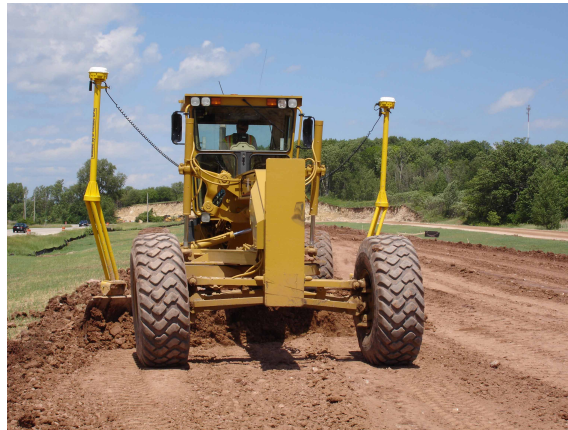
Figure 2.1: Picture of a Motor Grader with GNSS Antennae Attached for Use in AMG
