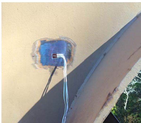
Figure 3.2-5. Triaxial strain gage at girder-knee joint.
