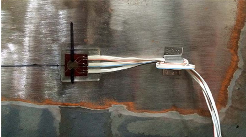
Figure 4.2-6. Triaxial strain gage at tail beam.
