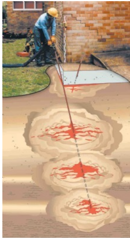
Figure 1.2: URETEK injection system ( www.uretek.com )
