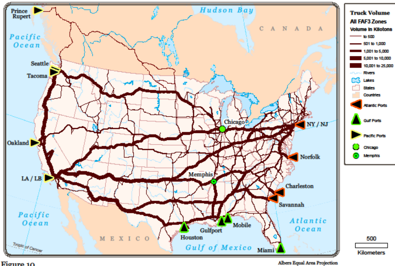
Figure 10 Results of Scenario 8: Truck Assignment (2019), All Freight Analysis Framework 3 [FAF3] Zones with Proportion of State Freight Volume by Population Proportion in each State. Modeling after Panama Canal expansion but before Prince Rupert expansion.
