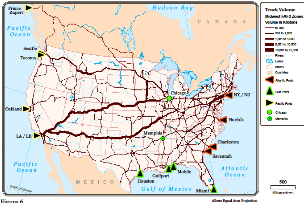
Figure 6 Results of Scenario 4: Truck Assignment (2012), Midwest Freight Analysis Framework 3 [FAF3] Zones with Proportion of State Freight Volume by Numbers of FAF3 Zones in each State. Modeling before Panama Canal expansion and before Prince Rupert expansion.
