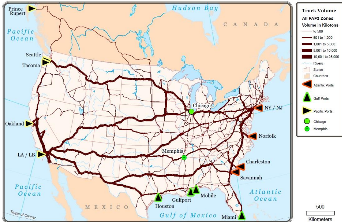
Figure 39 Result of Scenario 1: Truck Assignment (2012), All Freight Analysis Framework 3 [FAF3] Zones with Proportion of State Freight Volume by Number of FAF3 Zones in each State. Modeling before Panama Canal expansion and before Prince Rupert expansion.
