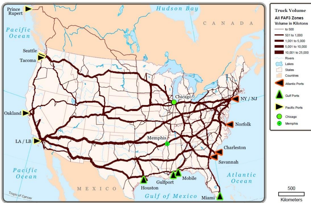
Figure 47 Result of Scenario 9: Truck Assignment (2020), All Freight Analysis Framework 3 [FAF3] Zones with Proportion of State Freight Volume by Population Proportion in each State. Modeling after Panama Canal expansion and Prince Rupert expansion.
