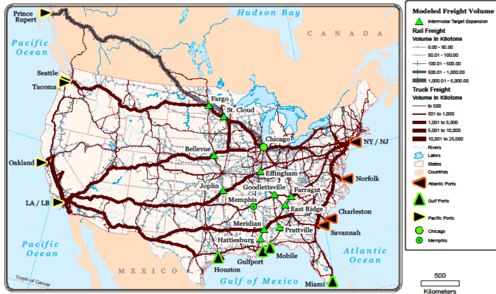
Results of Scenario 1: Freight Assignment (2012): All Freight Analysis Framework 3 [FAF3] Zones with Volume by numbers of FAF3 Zones in the State. Showing Intermodal locations (triangles) that are best suited near the CFIRE states because they are under 100,000 population, have intermodal capability, and will see a significant increase in volume due to port expansions.
