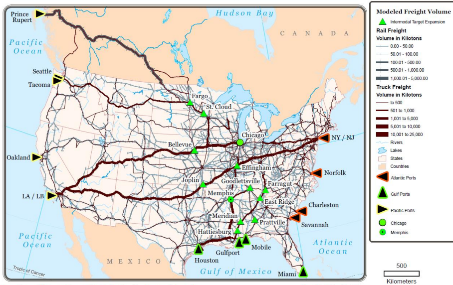
Results of Scenario 11: Freight Assignment (2019): Midwest Freight Analysis Framework 3 [FAF3] Zones with Population Proportion of FAF3 Zones in the State. Showing Intermodal locations (triangles) that are best suited near the CFIRE states because they are under 100,000 population, have intermodal capability, and will see a significant increase in volume due to port expansions.
