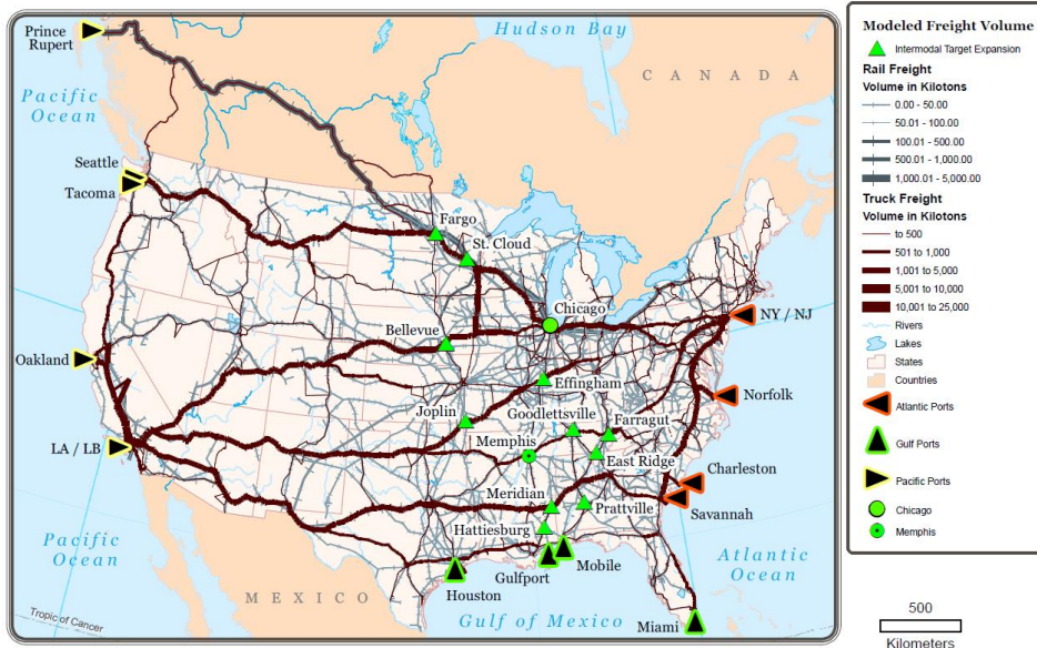
Results of Scenario 7: Freight Assignment (2012): All Freight Analysis Framework 3 [FAF3] Zones with Population Proportion of FAF3 Zones in the State. Showing Intermodal locations (triangles) that are best suited near the CFIRE states because they are under 100,000 population, have intermodal capability, and will see a significant increase in volume due to port expansions.
