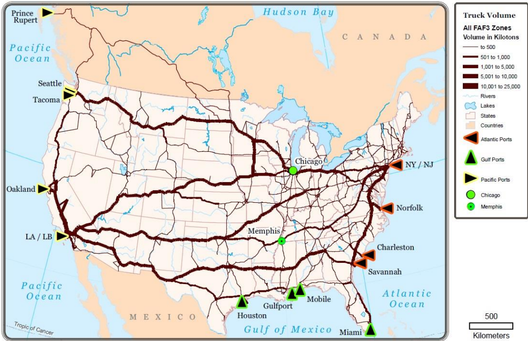
Figure 45 Result of Scenario 7: Truck Assignment (2012), All Freight Analysis Framework 3 [FAF3] Zones with Proportion of State Freight Volume by Population Proportion in each State. Modeling before Panama Canal expansion and before Prince Rupert expansion.
