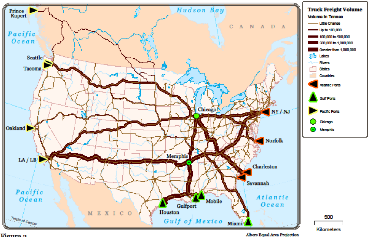
Figure 3 Scenario 3: 85% of forecasted container freight flows in 2020 from 13 US ports to Memphis and Chicago markets via trucks [Forecasted container freight flows for 2020 was received from individual port studies].
