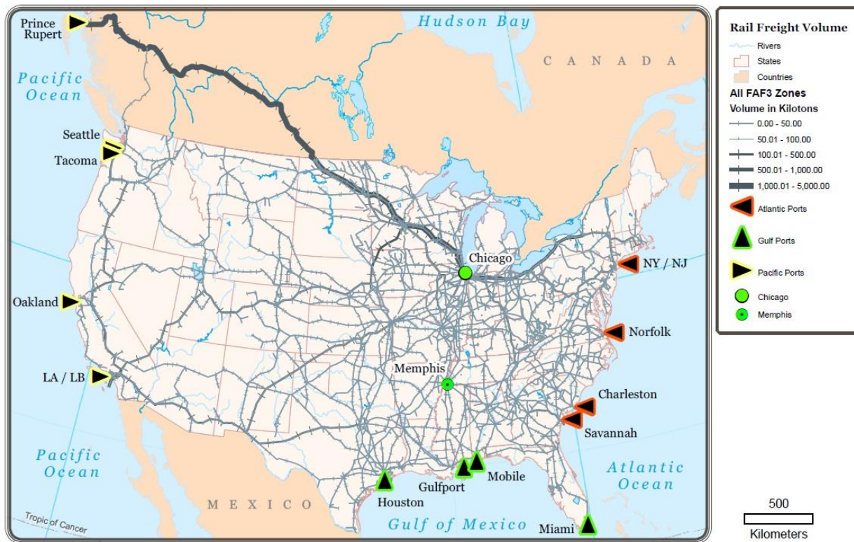
Figure 51 Result of Scenario 1: Railroad Assignment (2012), All Freight Analysis Framework [FAF3] Zones with Proportion of State Freight Volume by Numbers of FAF3 Zones in Each State. Modeling before Panama Canal expansion and before Prince Rupert expansion.
