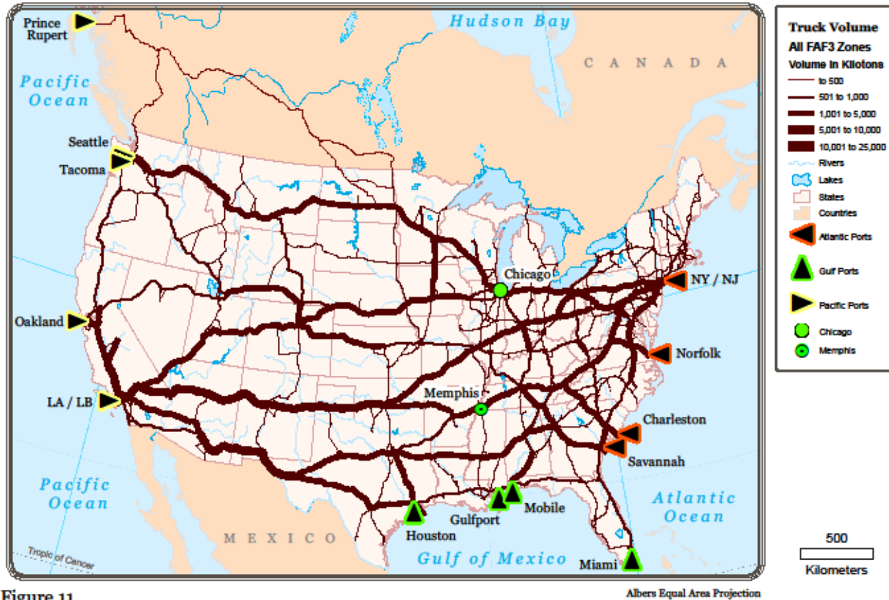
Figure 11 Results of Scenario 9: Truck Assignment (2020), All Freight Analysis Framework 3 [FAF3] Zones with Proportion of State Freight Volume by Population Proportion in each State. Modeling after Panama Canal expansion and after Prince Rupert expansion.
