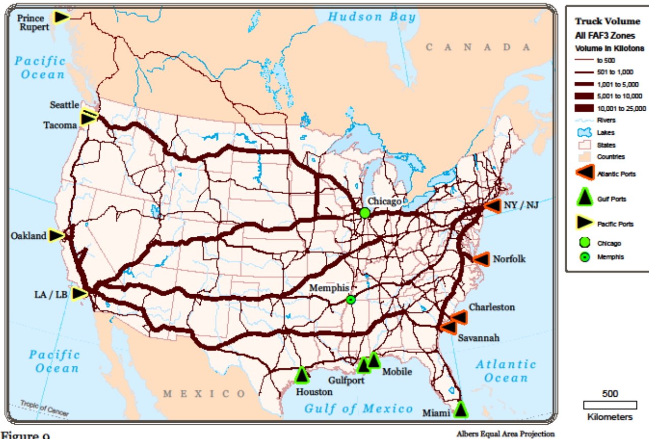
Figure 9 Results of Scenario 7: Truck Assignment (2012), All Freight Analysis Framework 3 [FAF3] Zones with Proportion of State Freight Volume by Population Proportion in each State. Modeling before Panama Canal expansion and before Prince Rupert expansion.
