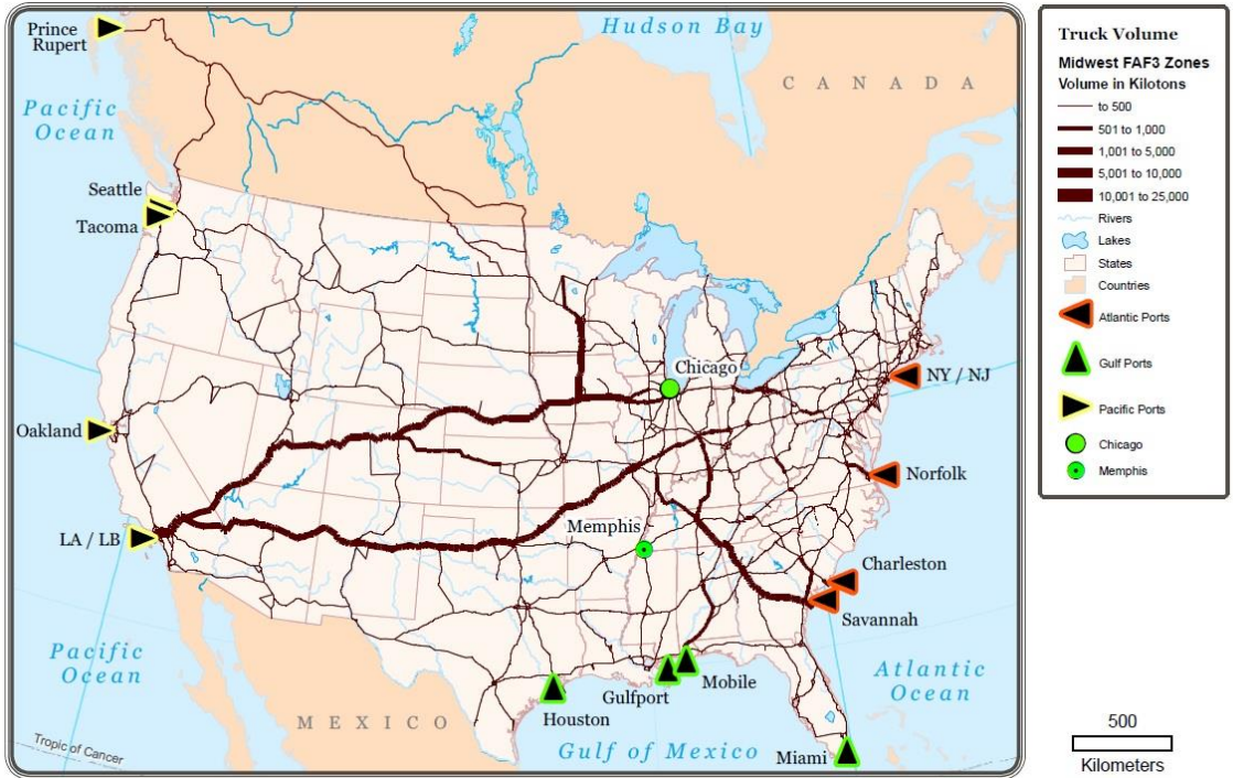
Figure 44 Result of Scenario 6: Truck Assignment (2020), Midwest Freight Analysis Framework 3 [FAF3] Zones with Proportion of State Freight Volume by Numbers of FAF3 Zones in each State. Modeling after Panama Canal and Prince Rupert expansion.
