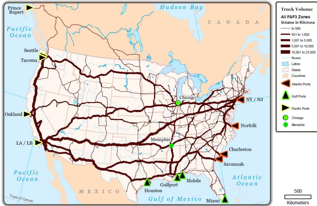
Figure 40 Result of Scenario 2: Truck Assignment (2019), All Freight Analysis Framework 3 [FAF3] Zones with Proportion of State Freight Volume by Number of FAF3 Zones in each State. Modeling after Panama Canal expansion, but before Prince Rupert expansion.
