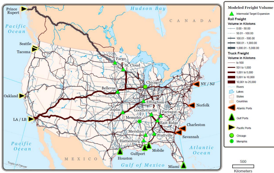
Results of Scenario 12: Freight Assignment (2020): Midwest Freight Analysis Framework 3 [FAF3] Zones with Population Proportion of FAF3 Zones in the State. Showing Intermodal locations (triangles) that are best suited near the CFIRE states because they are under 100,000 population, have intermodal capability, and will see a significant increase in volume due to port expansions.
