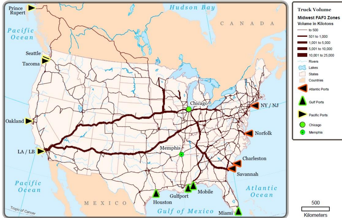
Figure 50 Result of Scenario 12: Truck Assignment (2020), Midwest Freight Analysis Framework 3 [FAF3] Zones with Proportion of State Freight Volume by Population Proportion in each State. Modeling after Panama Canal expansion and Prince Rupert expansion.
