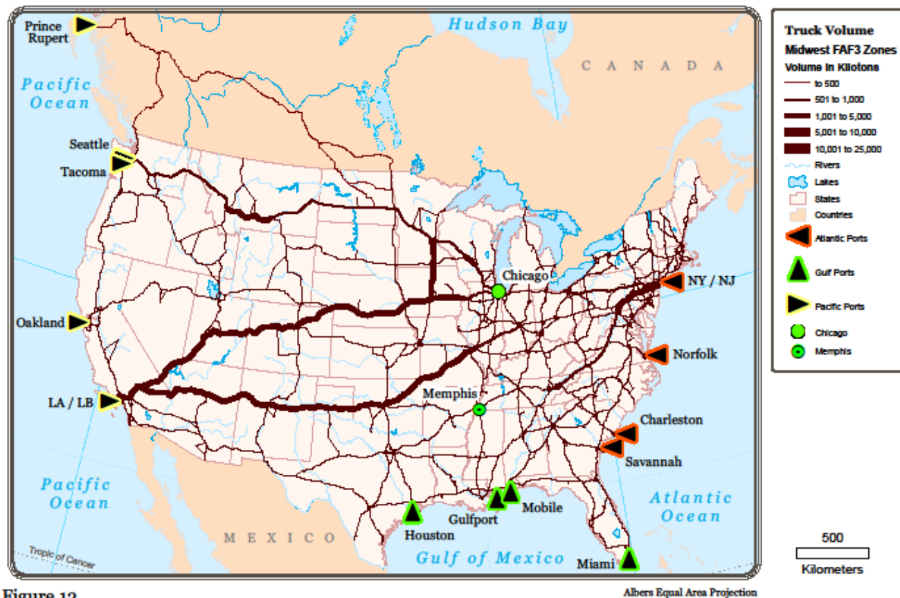
Figure 12 Results of Scenario 10: Truck Assignment (2012), Midwest Freight Analysis Framework 3 [FAF3] Zones with Proportion of State Freight Volume by Population Proportion in each State. Modeling before Panama Canal expansion and before Prince Rupert expansion.
