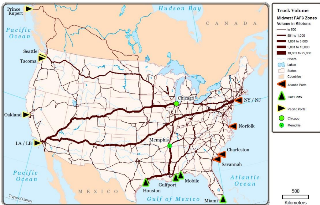
Figure 49 Result of Scenario 11: Truck Assignment (2019), Midwest Freight Analysis Framework 3 [FAF3] Zones with Proportion of State Freight Volume by Population Proportion in each State. Modeling after Panama Canal expansion, but before Prince Rupert expansion.
