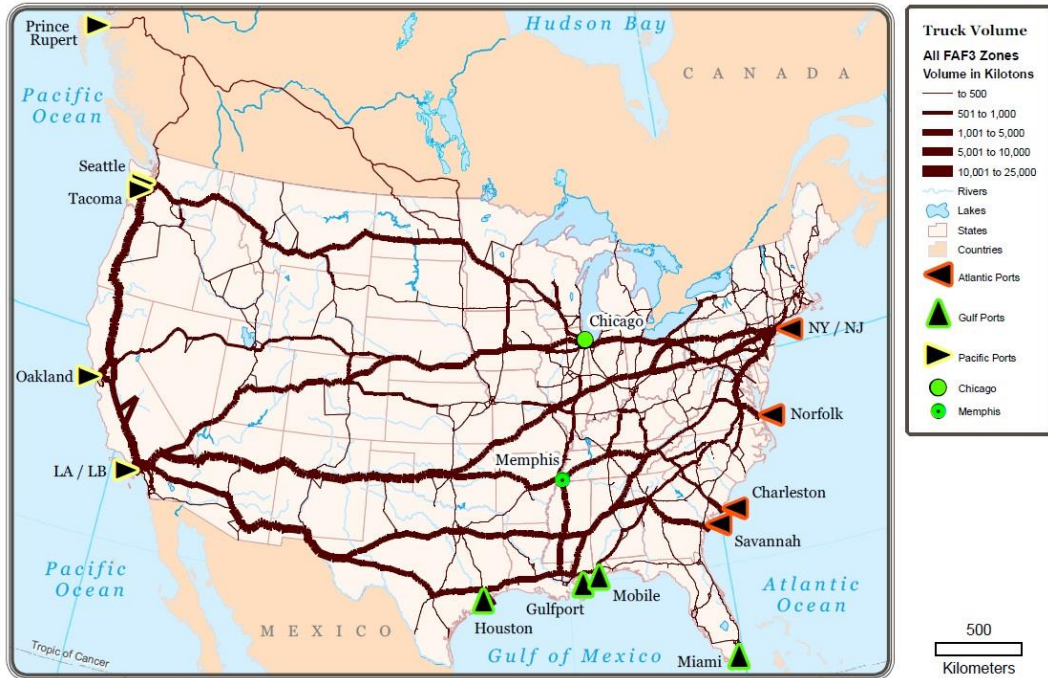
Figure 46 Result of Scenario 8: Truck Assignment (2019), All Freight Analysis Framework 3 [FAF3] Zones with Proportion of State Freight Volume by Population Proportion in each State. Modeling after Panama Canal expansion, but before Prince Rupert expansion.
