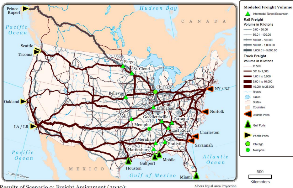
Results of Scenario 9: Freight Assignment (2020): All Freight Analysis Framework 3 [FAF3] Zones with Population Proportion of FAF3 Zones in the State. Showing Intermodal locations (triangles) that are best suited near the CFIRE states because they are under 100,000 population, have intermodal capability, and will see a significant increase in volume due to port expansions.
