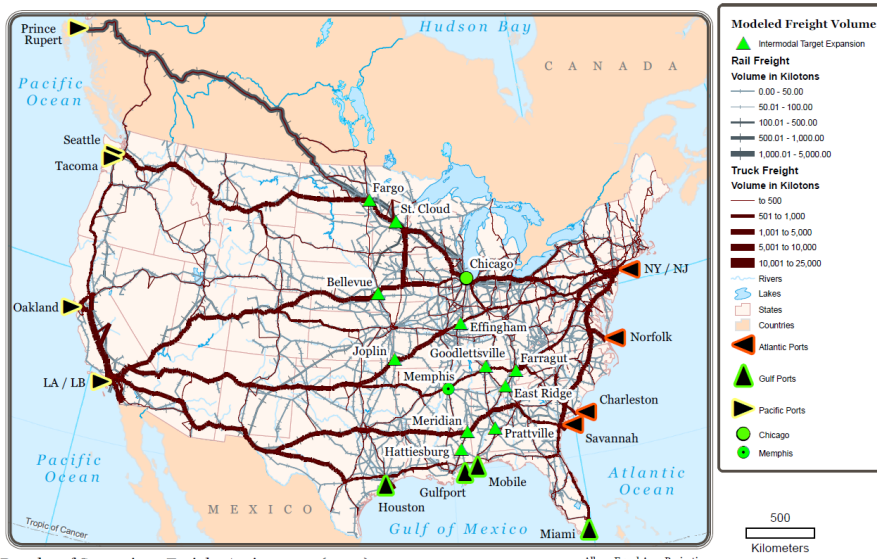
Results of Scenario 1: Freight Assignment (2012): All Freight Analysis Framework 3 [FAF3] Zones with Volume by numbers of FAF3 Zones in the State. Showing Intermodal locations (triangles) that are best suited near the CFIRE states because they are under 100,000 population, have intermodal capability, and will see a significant increase in volume due to port expansions.
