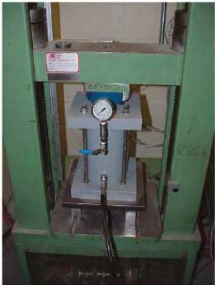
Figure 2.12: Water Permeability Test setup (Banthia et al., 2005)
