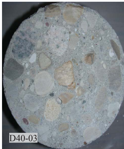
Figure 3.38: Surface conditions of samples D40-03/04
