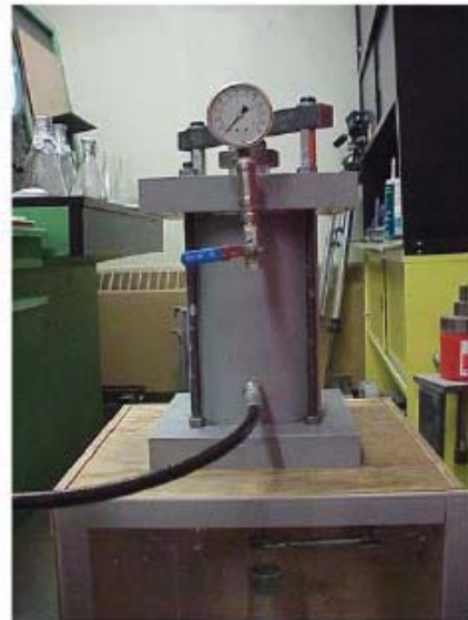
Figure 2.12: Water Permeability Test setup (Banthia et al., 2005)
