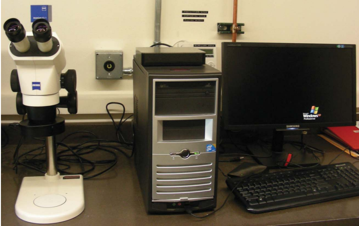
Figure 4.1: Optical microscope used to observe microcracks in samples
