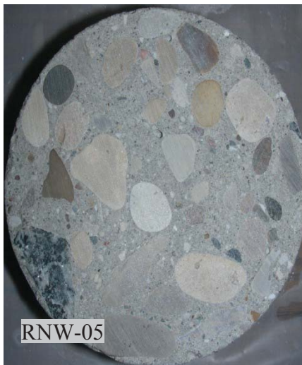
Figure 3.26: Surface conditions of reference samples RNW-05/06
