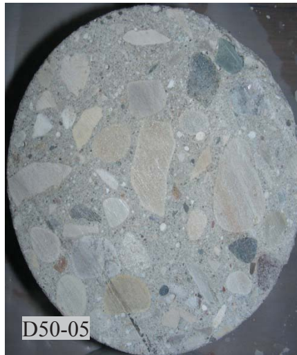
Figure 3.47: Surface conditions of samples D50-05/06
