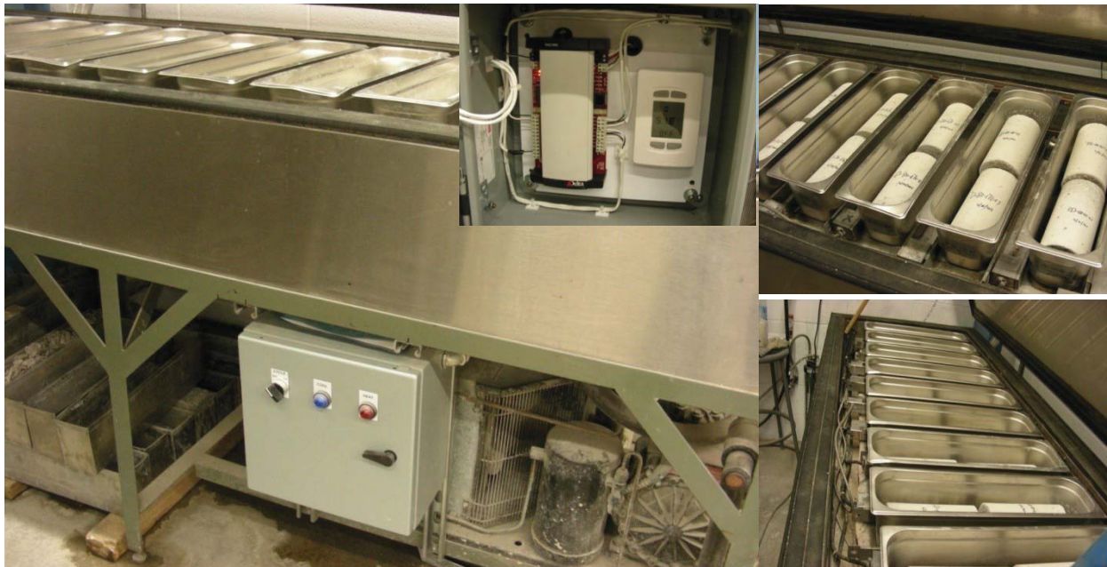
Figure 3.4: Modified HM-12 Freeze-thaw Test Chamber
