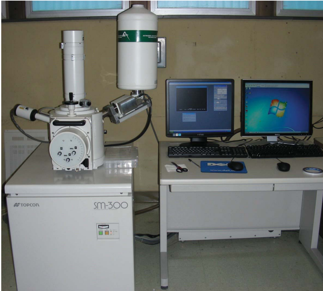
Figure 4.6: Using (Topcon SM300) SEM techniques to capture the microstructures of concrete
