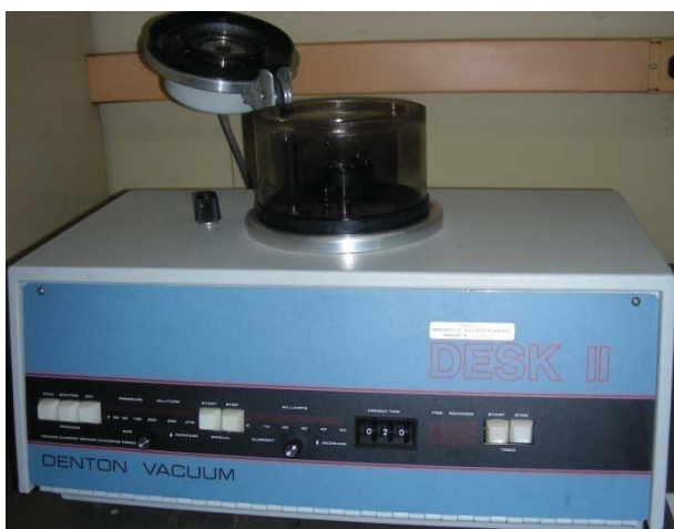
Figure 4.8: Denton Desk II Sputter Coater and coated samples
