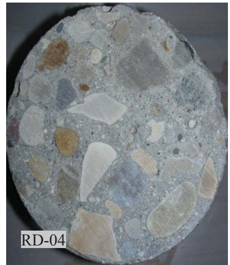
Figure 3.31: Surface conditions of reference samples RD-03/04
