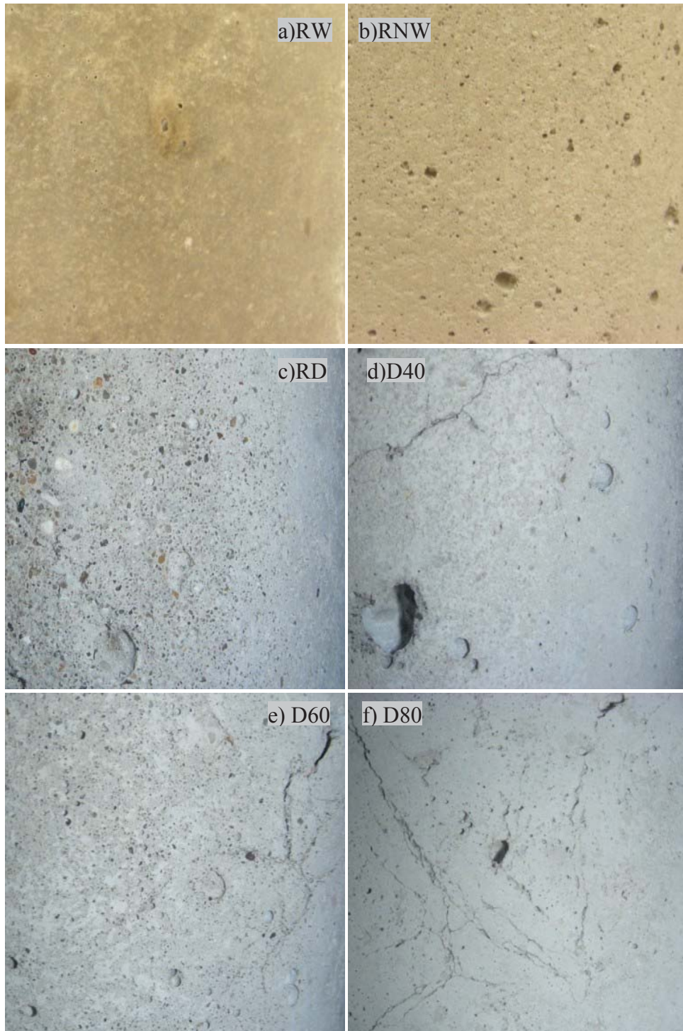
Figure 3.6: Typical surface conditions after F/T cycles
