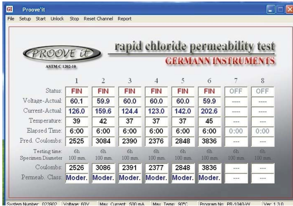
Figure 3.14: PROOVE'it© software in PC screen to run the test and acquire the data
