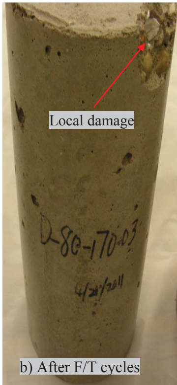
Figure 3.68: Surface conditions of samples D80-05/06
