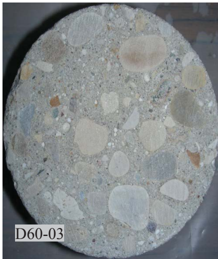
Figure 3.52: Surface conditions of samples D60-03/04
