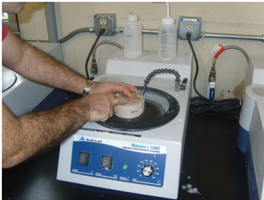
Figure 4.2: A semi-auto Grinder-Polisher used to polish samples
