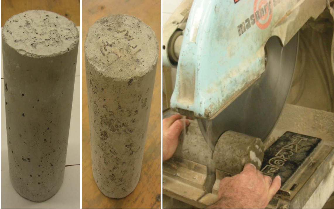
(a) before F/T cycles (b) after F/T cycles (c) cut 2-inch slice from a specimen
