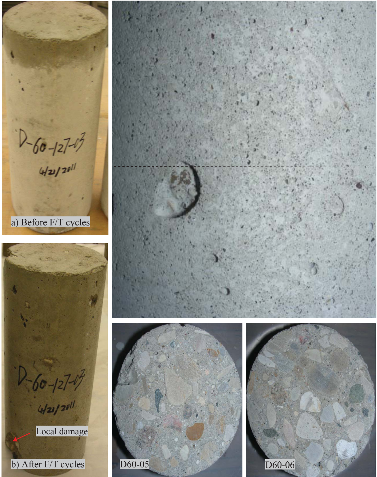
Figure 3.54: Surface conditions of samples D60-05/06
