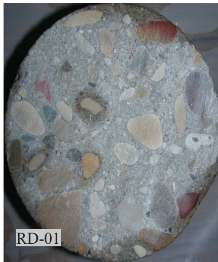
Figure 3.29: Surface conditions of reference samples RD-01/02
