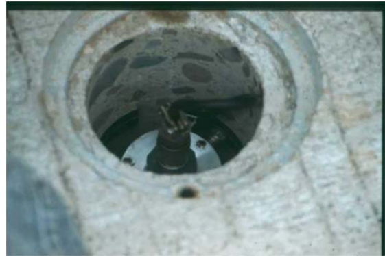
Figure 7.7: LVDT installed at MnROAD
