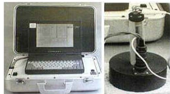
b. Installation of ECI corrosion meter (Virginia Technologies, Inc.).
