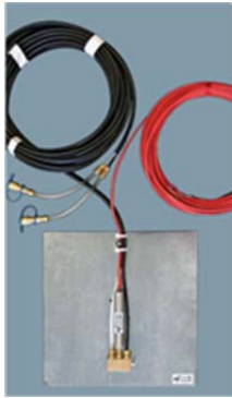
c. Vibrating Wire Liquid Settlement System and Typical Installation for Monitoring Settlement of Embankment ( http://www.rstinstruments.com )
