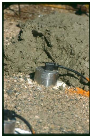
Figure 7.5: Tiltmeter installations at MnROAD
