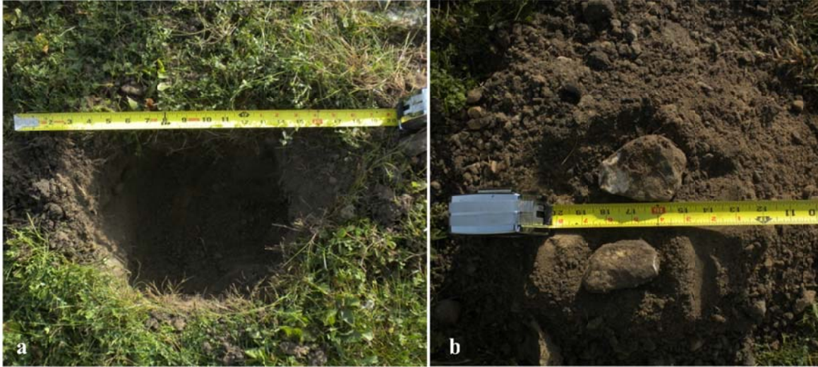
Figure 3.6. Exploration trench performed for CPTU2-05 at Long-13. Frame a. shows exploration trench and frame b. is the material excavated from the trench. Note the gravel size fill found at the near surface.
