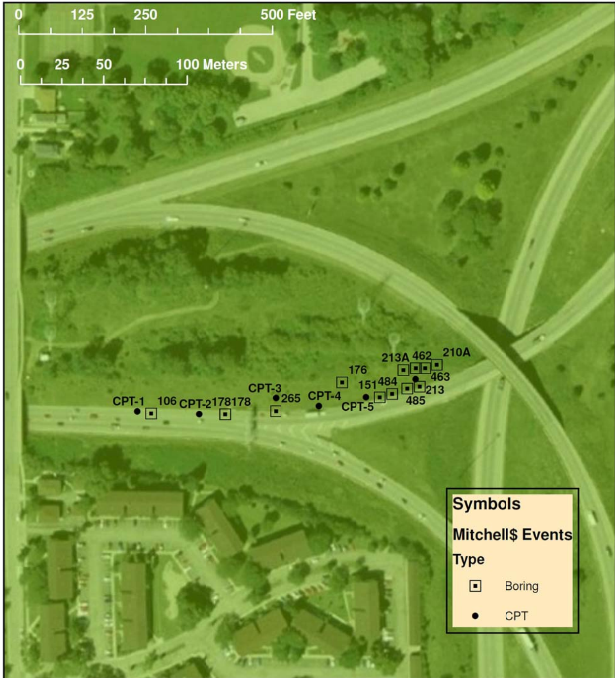
Figure 2.20. Location of WisDOT CPT tests and adjacent borings for Mitchell Interchange. Pressuremeter data available for Boring 178 and 210A. Wisconsin Quaternary geology adapted from data on previously published maps (Linebeck et al. 1983) Aerial photo from ESRI ArcGIS Online, World Imagery.
