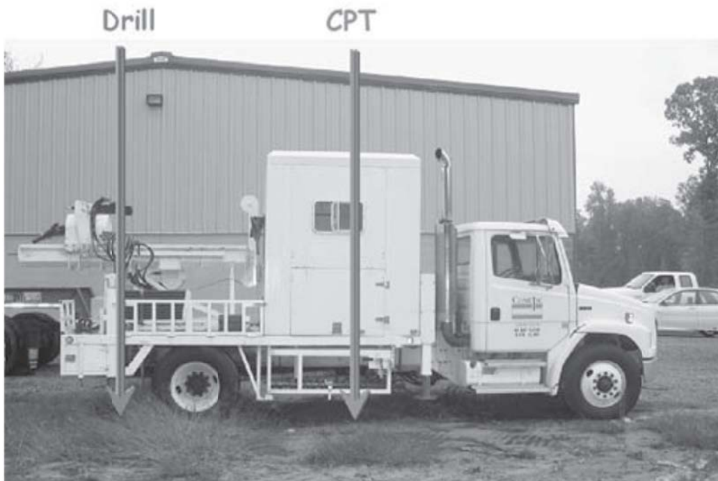
Figure 7.5. CPT rig with drilling capabilities (Mayne 2007)
