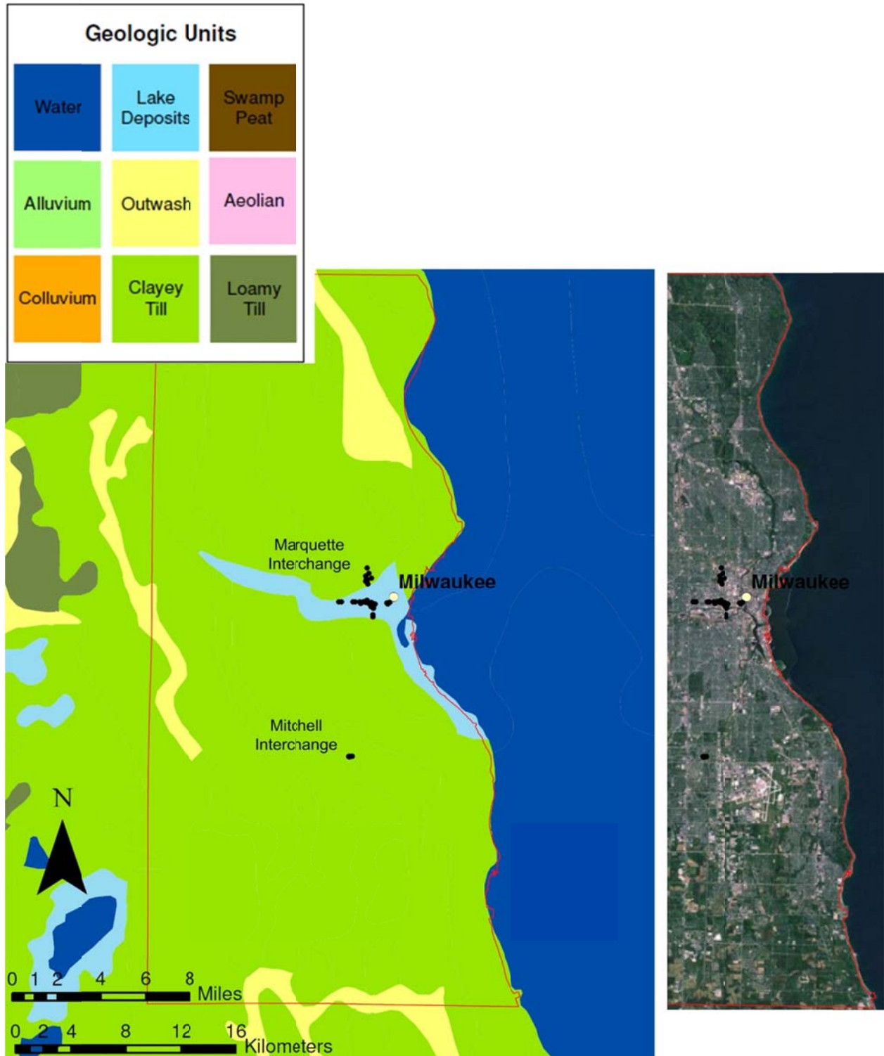
Figure 2.18. Location of WisDOT CPT sites from previous projects. Wisconsin Quaternary geology adapted from data on previously published maps (Linebeck et al. 1983) Aerial photo from ESRI ArcGIS Online, World Imagery.
