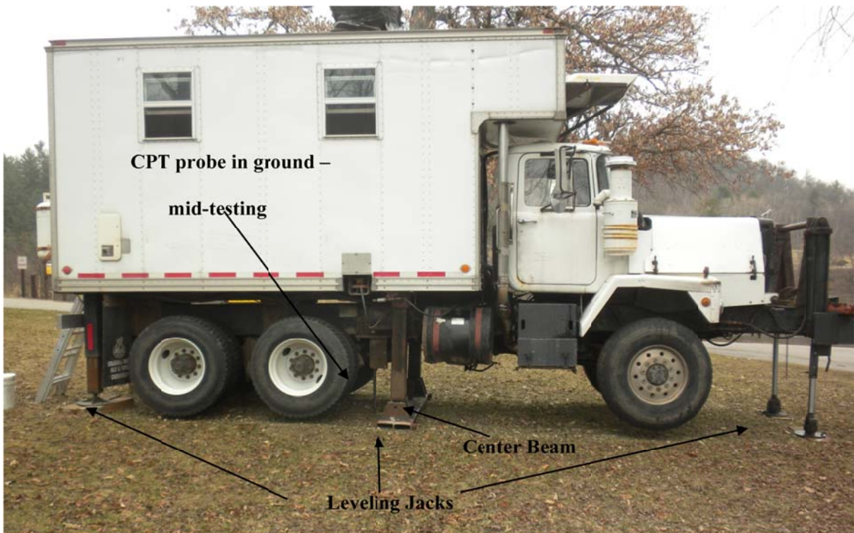
Figure 3.1. University of Wisconsin-Madison's 24-ton CPT truck setup at site DOT-3R. Note front and rear wheels are not in contact with the ground, so that all of the truck weight is suspended.
