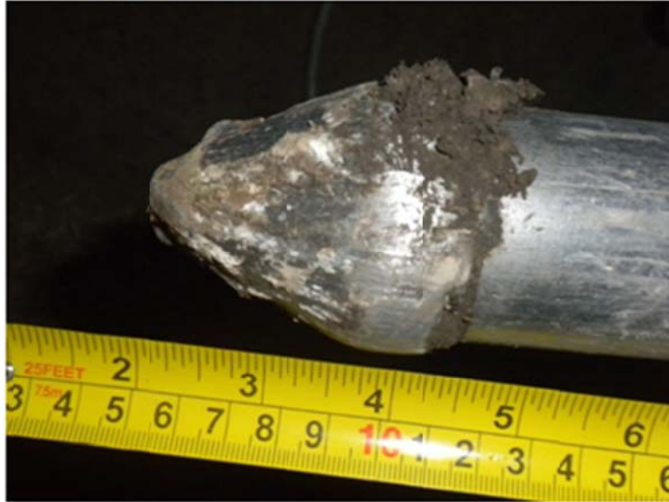
Figure 4.16. The dummy rod consists of a conical tip welded to a push rod with a 1.75 in outer diameter. The dummy push rod was used to check for near surface refusal and presence of gravel fill. Note white dust on tip from pulverized material.
