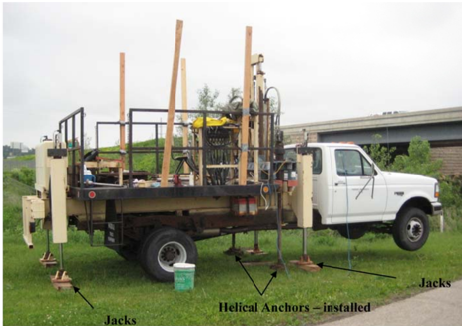
Figure 3.3. Purdue University's CPT truck setup on site at Long-10. Jacks for lifting truck and helical anchors are called out.
