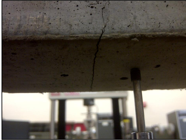
Figure 66: Single Crack Failure
