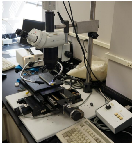
Figure 19: Investigation using Modified Point Count Procedure of ASTM C457
