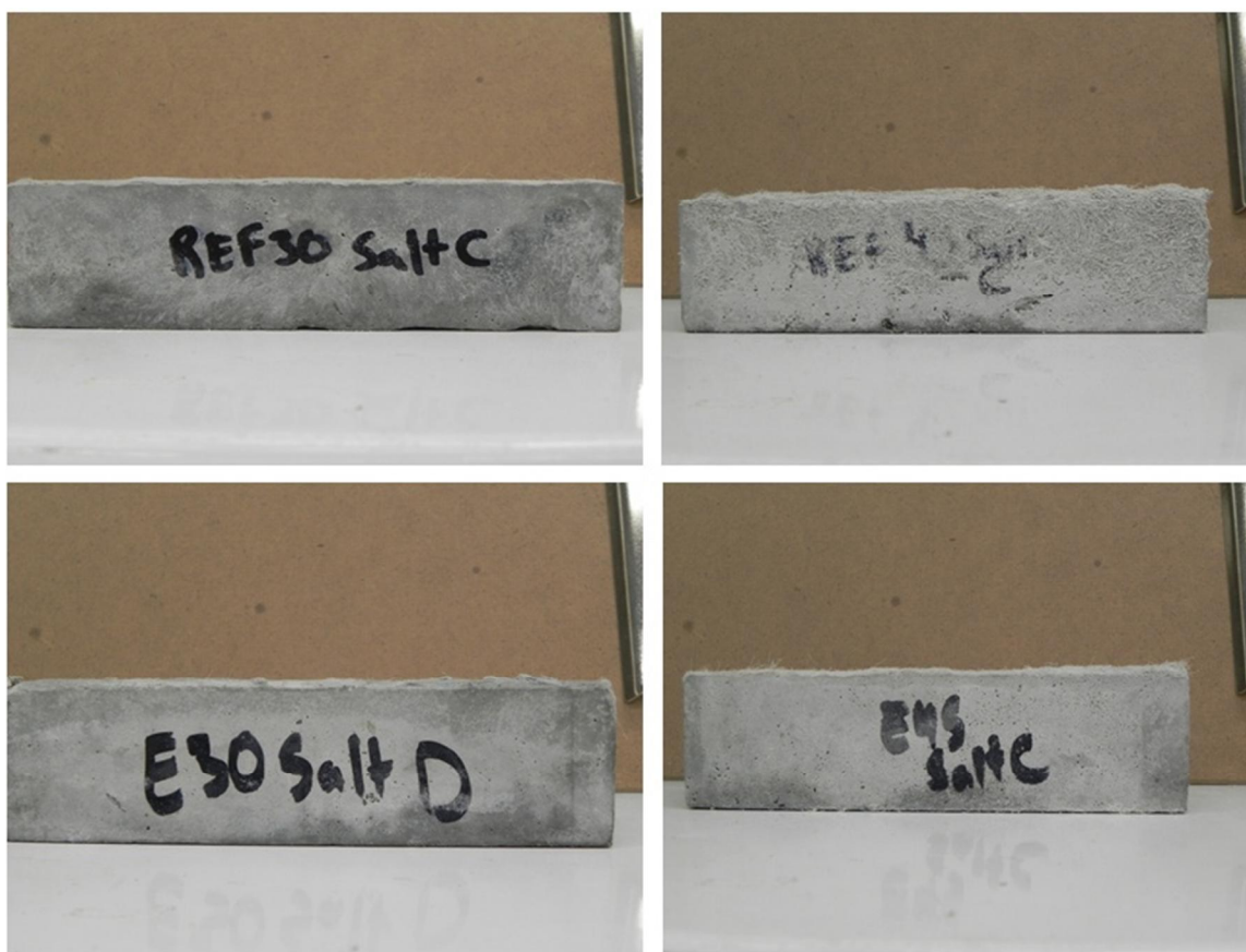
Figure 46: Surface Scaling of ECC/SECC after Freezing and Thawing Cycles
