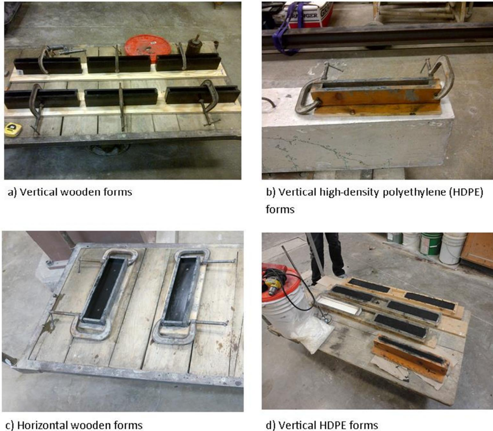
Figure 63: Different Formworks used for 1 x 3 x 15 in Beams
