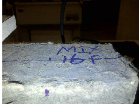
Figure 68: Rough Loading Surface from Horizontally Placed Molds
