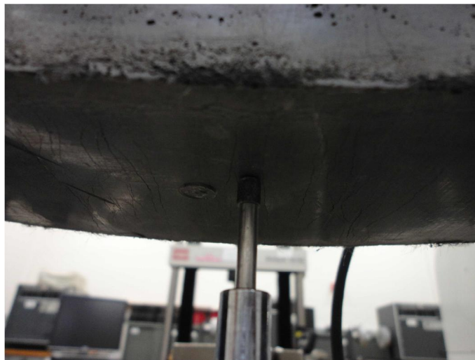
Figure 73: Steady-State Cracking Pattern of ECC
