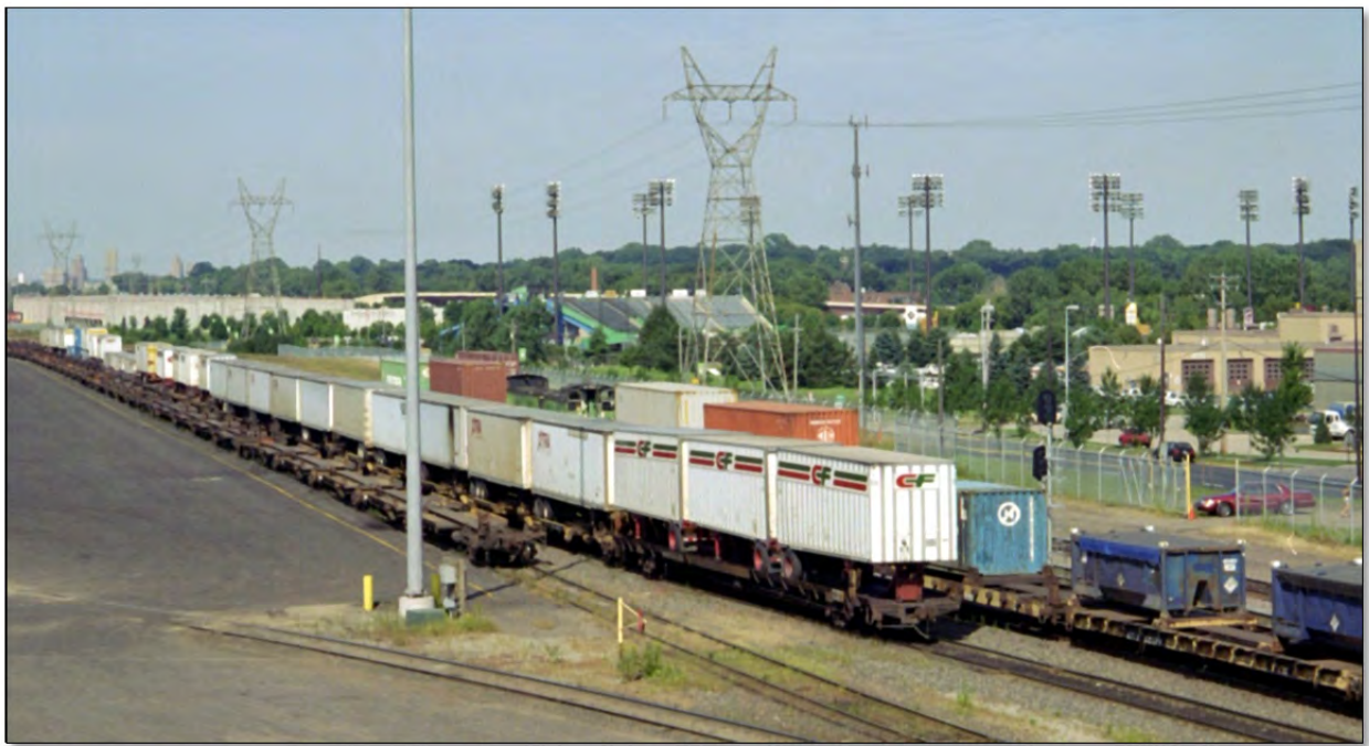
Figure 9: Trailer on Flat Car, May 2012 (Photo R.D. Stewart)
