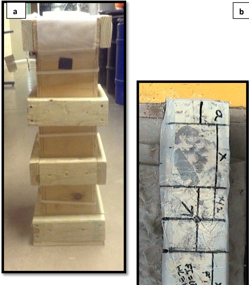
Figure 3.10 Picture of Beam Mold (a); Beam PSFB (b) after Injection
