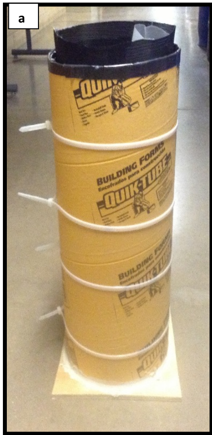
Figure 3.9 Cylindrical Mold (a), Cylindrical PSB (b) after Injection
