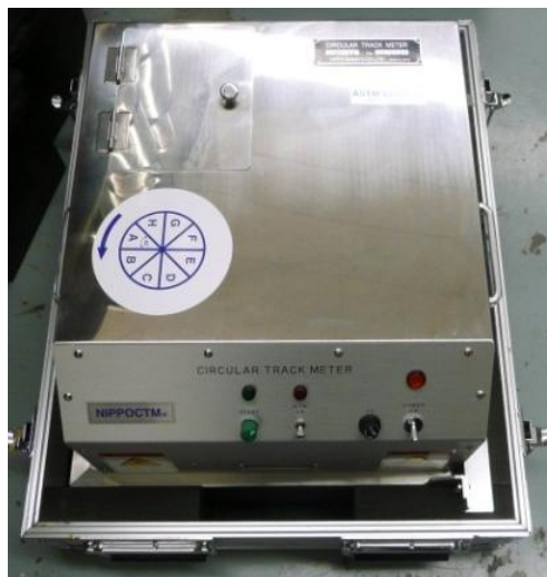
Figure 6. The Circular Track Meter (CTM) is used to evaluate pavement macro-texture.
