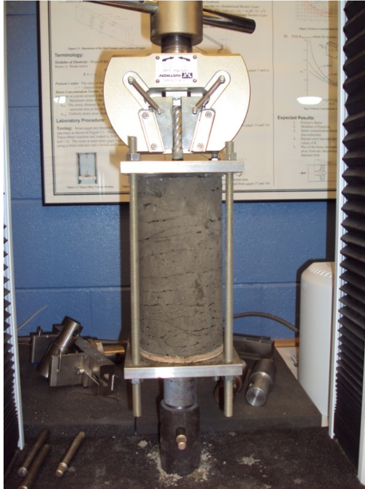
Figure 2.11: Pullout Test Type 1
