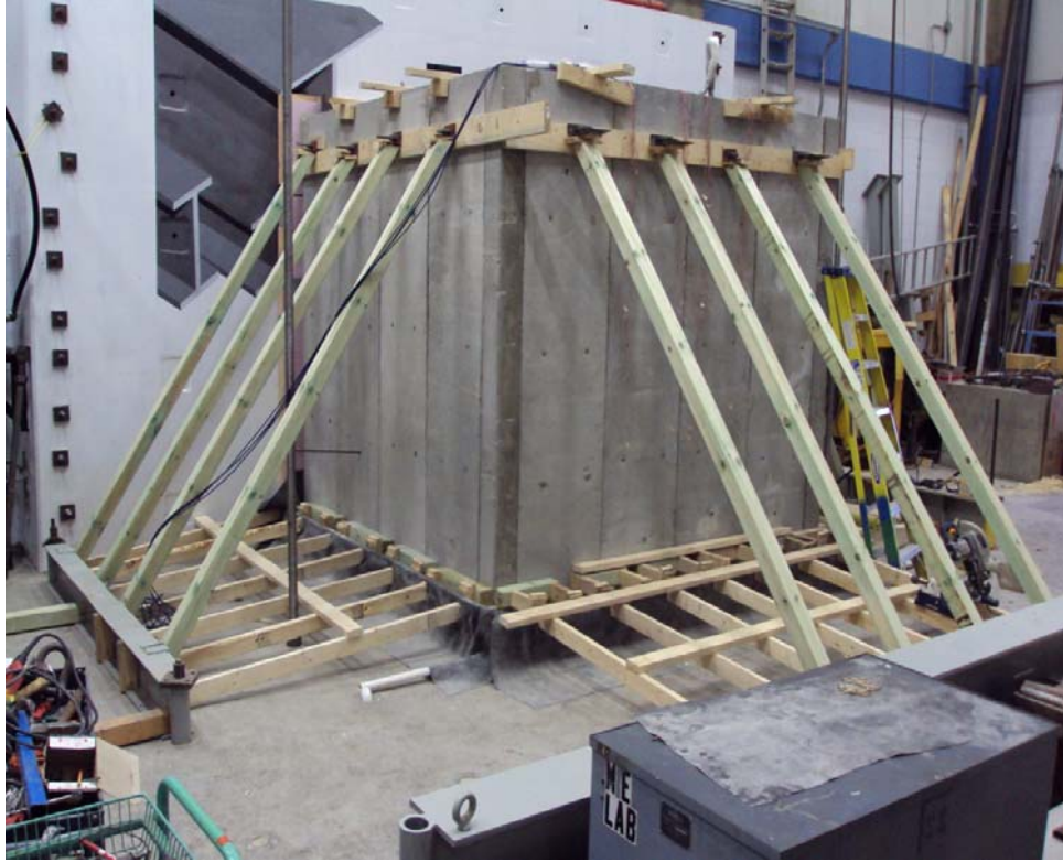
Figure 3.12: Temporary Lateral Support of Concrete Panels
