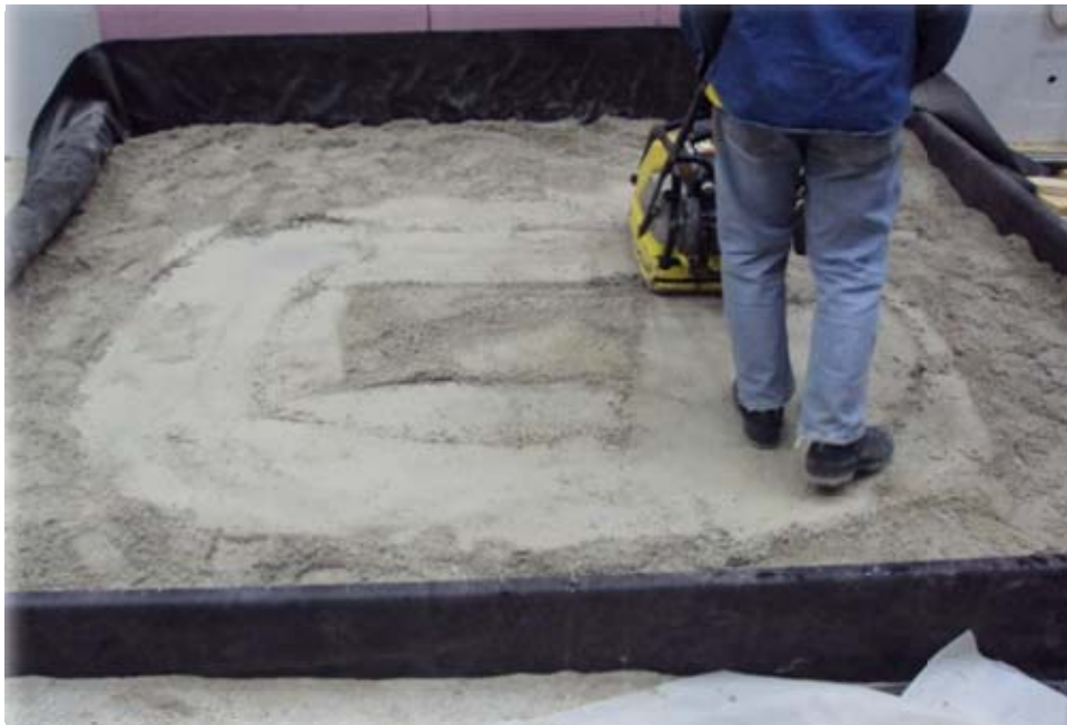
Figure 3.8: Compaction of the Base Soil Layer
