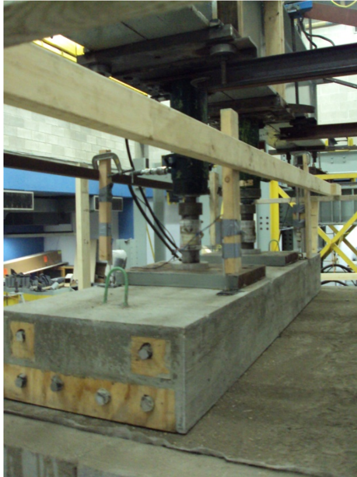
Figure 3.16: Reinforced Concrete Sill Placement
