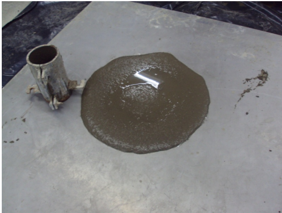
Figure 2.2: Standard Test Method for Flow Consistency of CLSM
