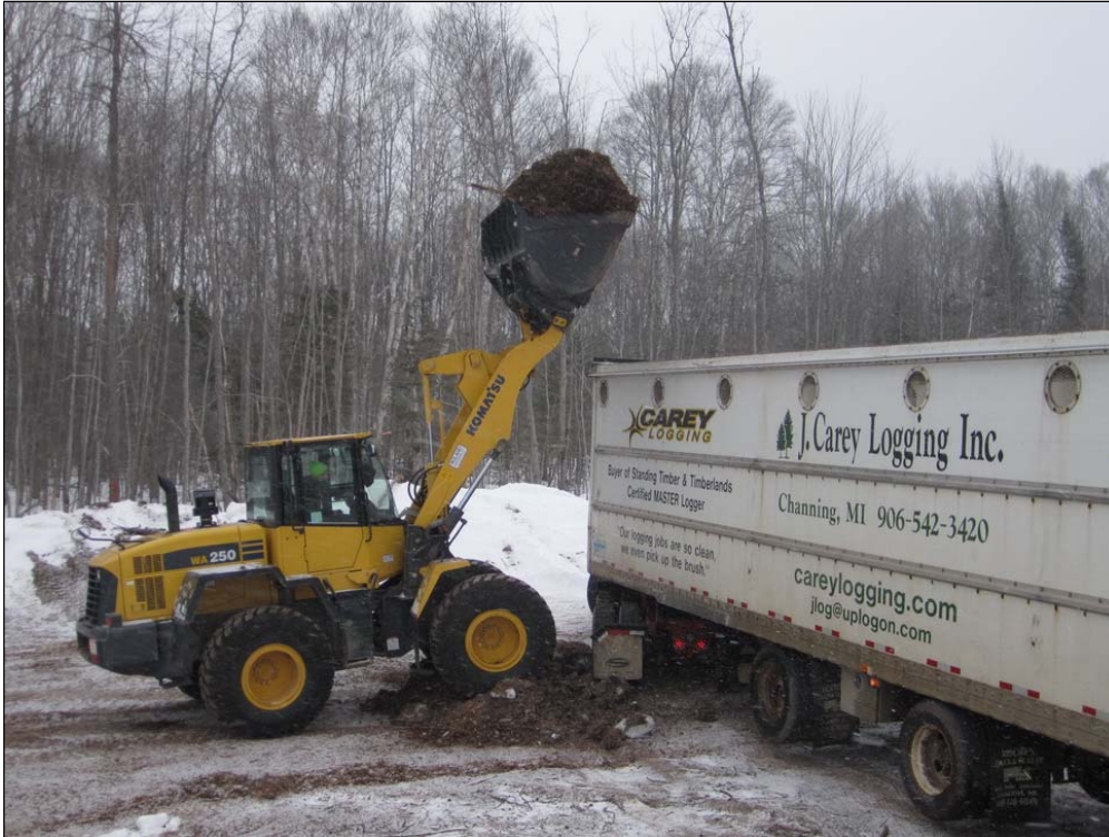
3.12.3 Loading the chip truck by using a front-end loader. A temporary chip pile beside the truck is used to help the loader reach over the truck lip (Photo by J. Vartiainen, Feb. 11)
