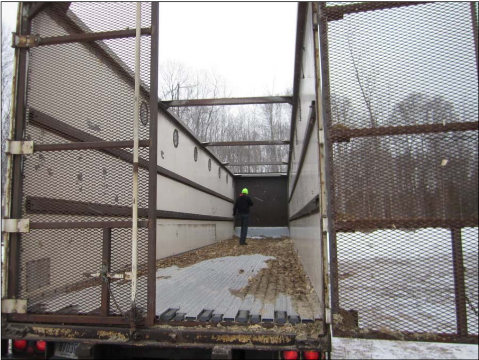
3.12.2 Inside of a chip truck prior to loading (Photo by J. Vartiainen, Feb. 11)
