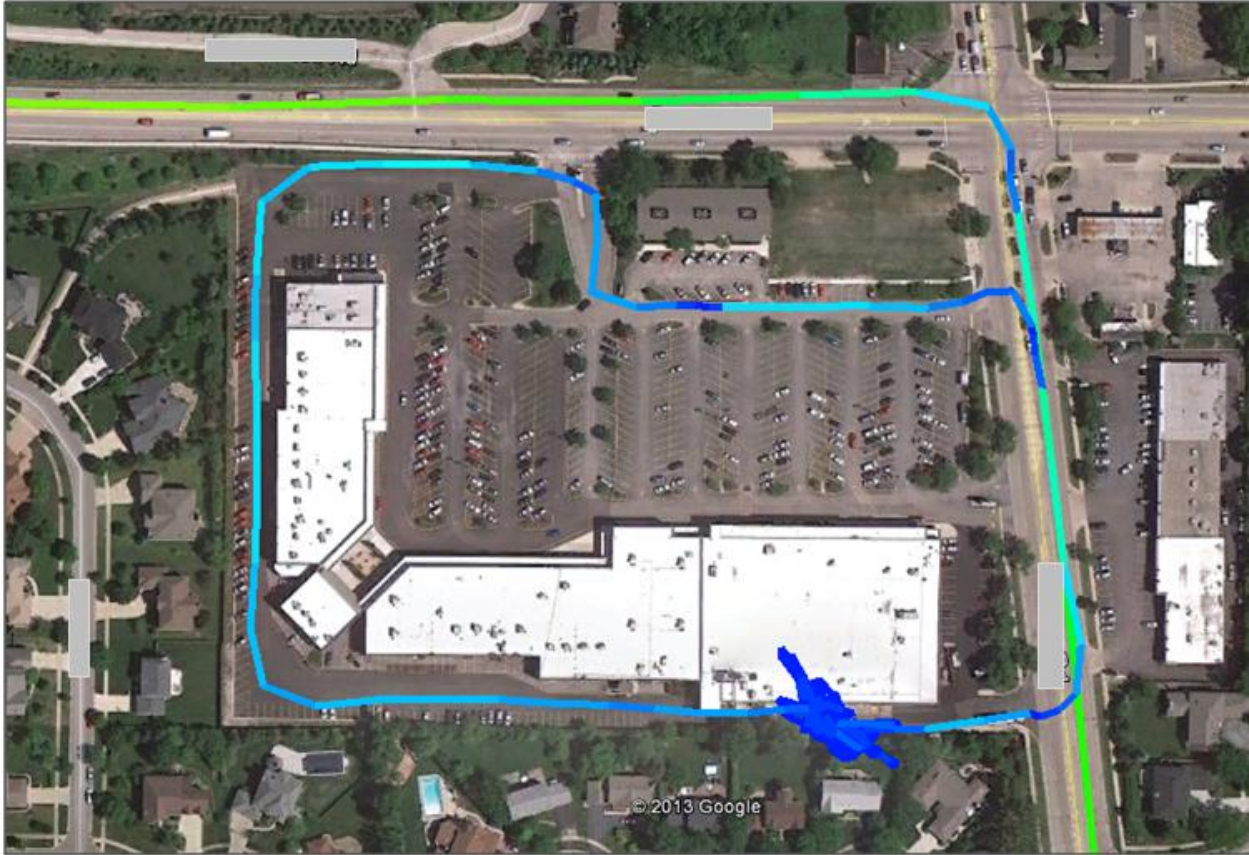
Figure 12: GPS Tracks of Truck Entering and Exiting a Scheduled Stop
