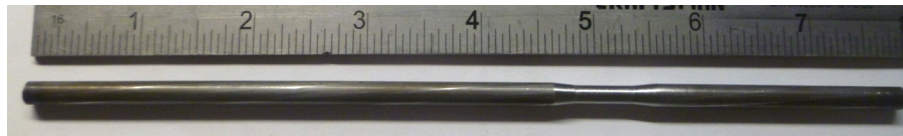
Figure-7. 1 Steel wire on lathe with reduced cross-section
