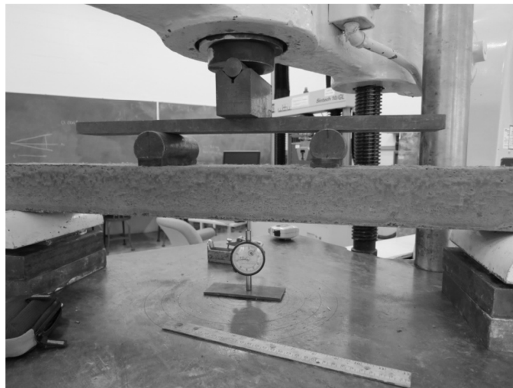
Figure 18: Flexural setup for 36-inch beams
