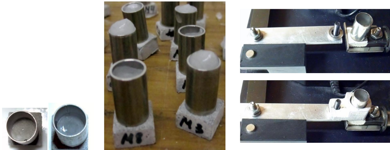
Figure 16: The specimen preparation for the ice adhesion tests (left and center) and the setup for the test (right)
