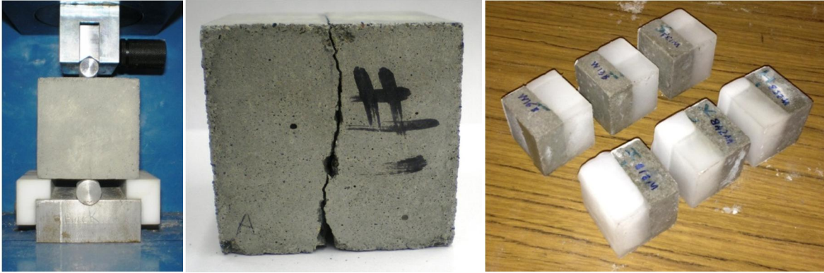
Figure 14: The set up for the specimen test (left), crushed specimens (center), and specimens treated with hydrophobic agent and bonded ice (right)
