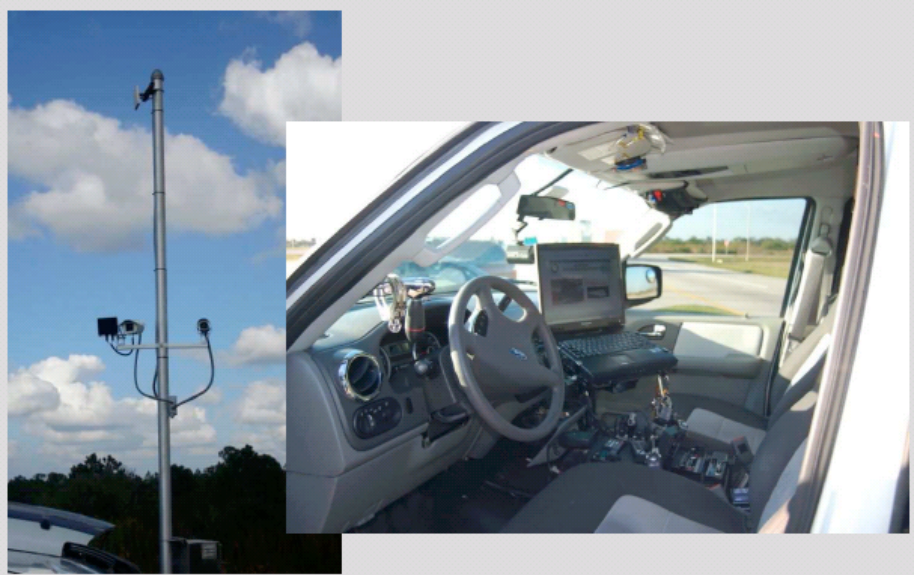
Figure 9.2 Virtual Weigh Station Transponder and In-Vehicle Computer
