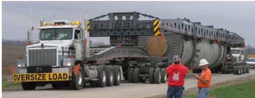
Figure 1-1. Special overload vehicle (from Perkins Motor Transport)
