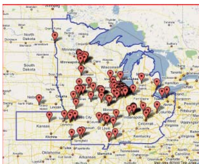
Survey markings showing truck parking problem areas in the Midwest
